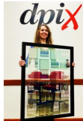
X-ray photo detector arrays for medical imaging on Gen 4.5 glass
