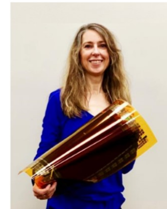
X-ray photo detector arrays for medical imaging on Gen 4.5 flexible substrate
