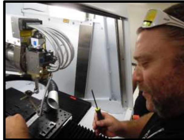
Adjusting the parts fixture
