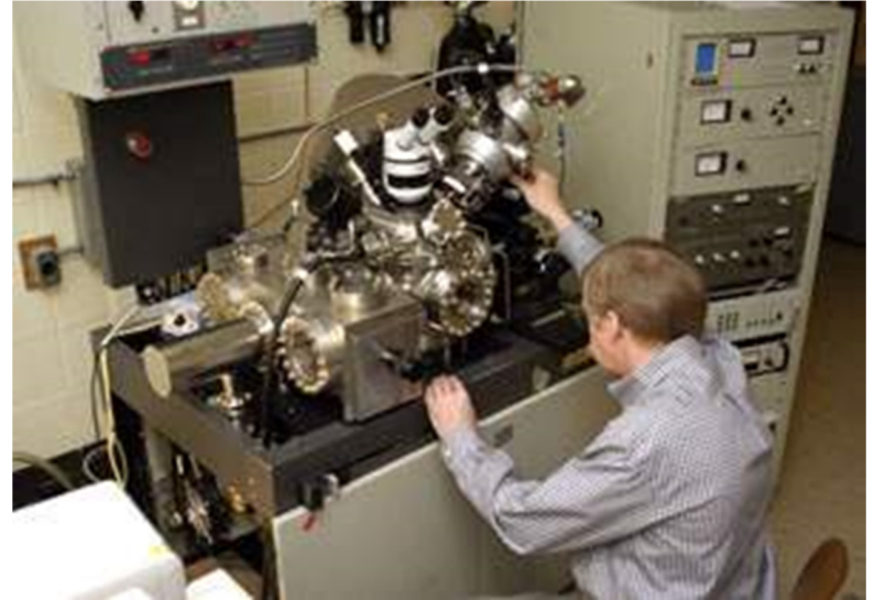
Vintage SSX-100 XPS Spectrometer - University of Toronto
